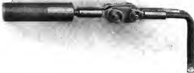
Fig. 7—The separable joint connected up, ready for use
